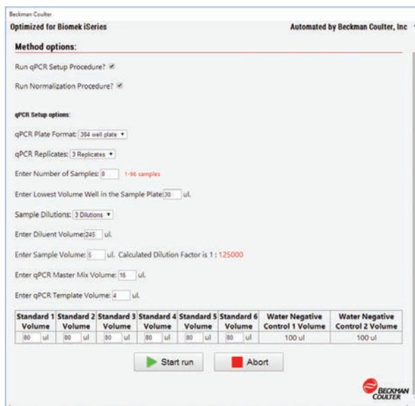
Figure 4. Example of Method Options Selector (MOS) for the KAPA qPCR Method. User can select what section of the method to be run, number of samples, plate type, replicates and details about the standards.
