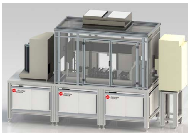
Fig. 2. Representation of the integrated cell culture system used to automate the differentiation of mESCs.
